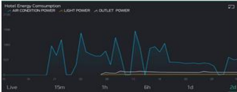
Figure 4: Example of a hotel room (35 sq.m.) energy consumption profile (W) of air conditioner, lighting, and an outlet for two days period
